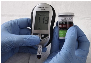
FIGURE 38-17 The code on the bottle of reagent (test) strips is compared to the code on the glucometer.
