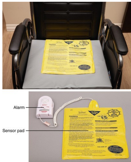
FIGURE 14-3 A position change alarm. This alarm has a sensor pad. The alarm sounds when the person moves off of the pad.
