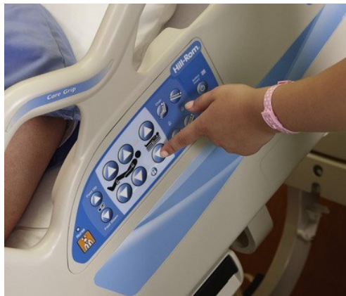
FIGURE 21-6 Controls for staff use are on the outer part of the rail. (Courtesy © Hill-Rom Services, Inc. Reprinted with permission. All rights reserved.)
